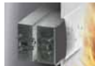
The intumescent layer within the box expands as the temperature increases filling the metal box cavity.
